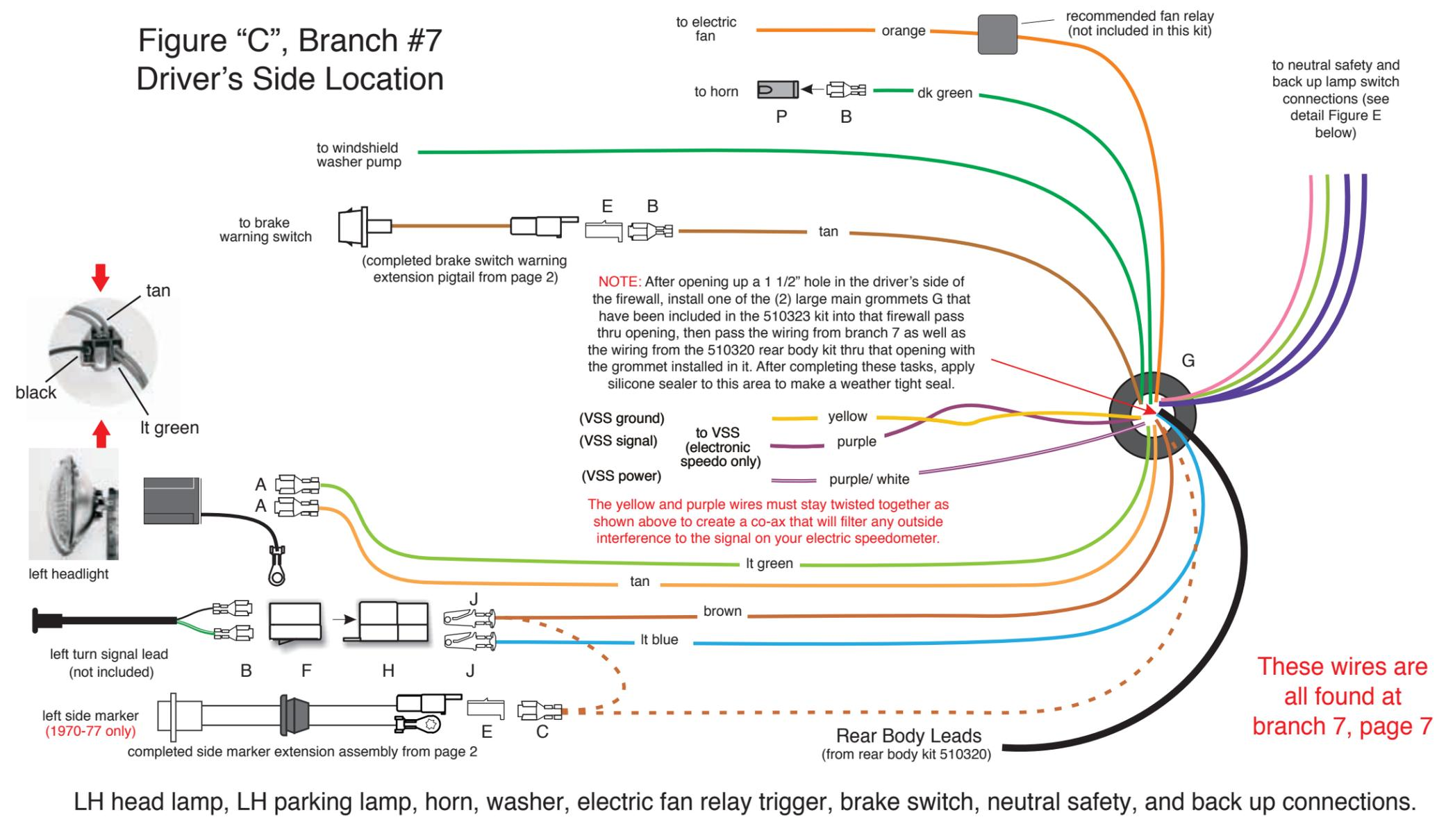
LH head lamp, LH parking lamp, horn, washer, electric fan relay trigger, brake switch, neutral safety, and back up connections.
