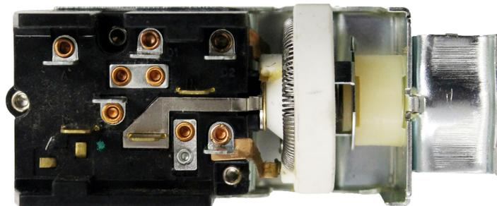
1. Install the new switch into your dash using the original bezel and nut. It will be necessary too cut the shaft for a nice custom installation.
