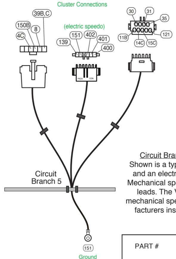
Note: Your VSS Signal and Ground wires have been twisted together from the factory and must remain this way to shield out any outside electrical interference that may create an issue with the proper operation of your electric speedometer.
