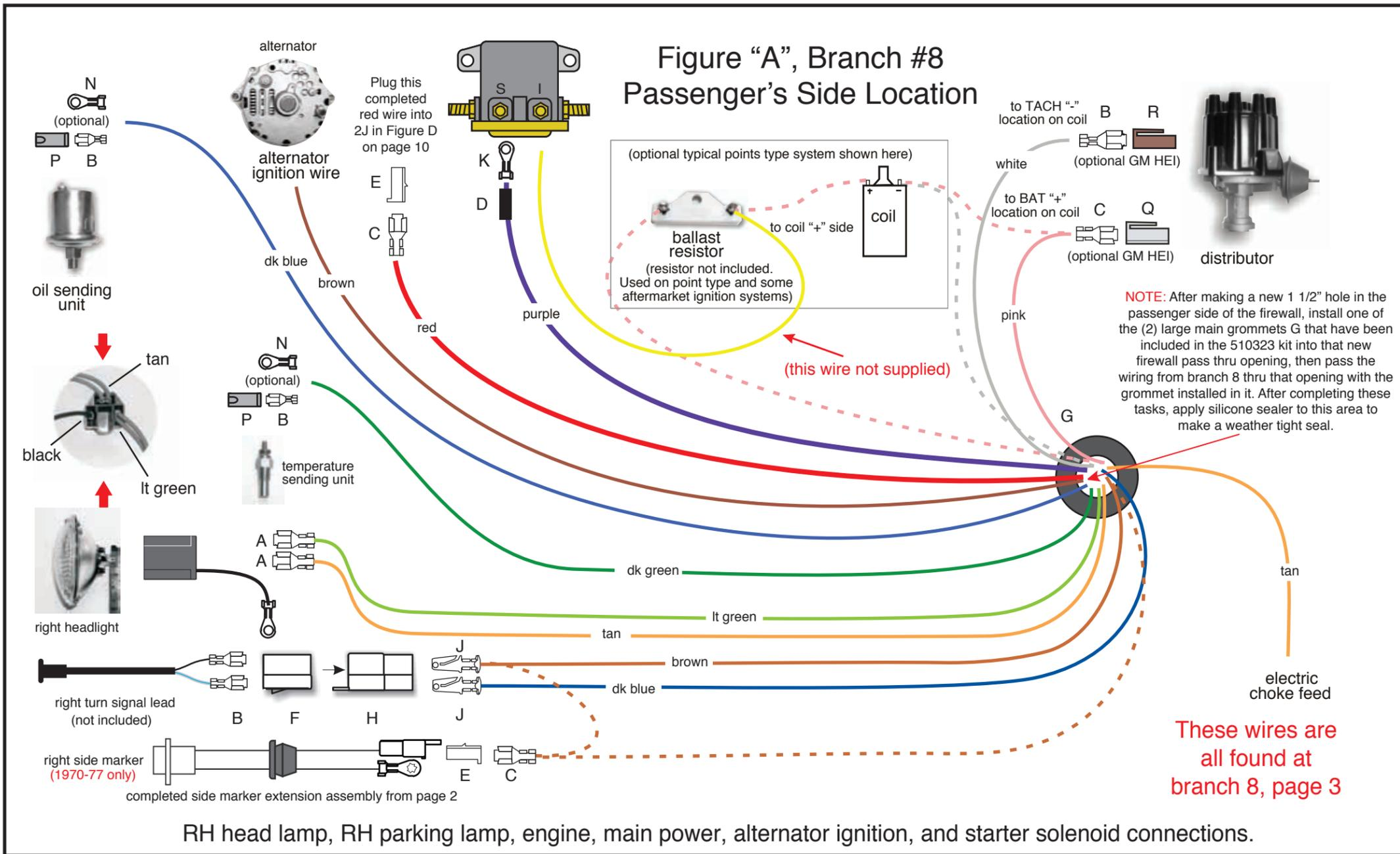
**NOTE:** The terminals and connectors listed on this page and denoted with **UPPER CASE LETTERS** to help you complete the various connections to your lamps, engine connections, switches, etc. can be found in your loose piece clamp, grommet, and parts kit, P/N 510323.
