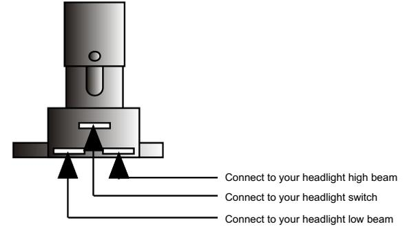
Connect the Dimmer Switch wires as shown above.
